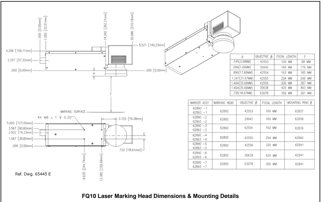
FQ10 Laser Marking Head Dimensions & Mounting Details
